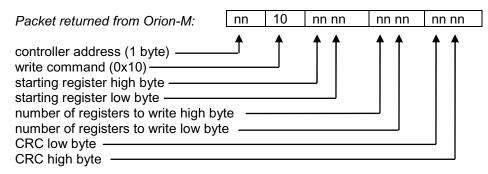
Example: Set the profile start step to 1 (register 14) and start the profile (value of 8 in register 15) on the
