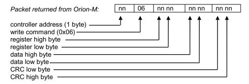
Example: Write register 67 (loop 3 setpoint) of controller at address one configured with no decimal point to
