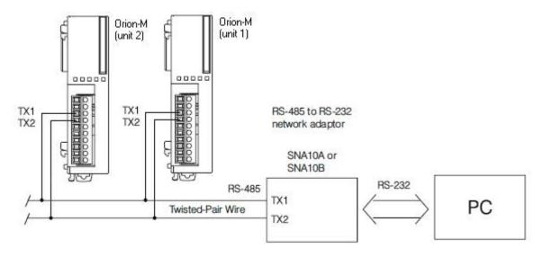
NOTE: When using shielded twisted-pair cable, be sure to ground only when end of the cable, preferably at the RS232 to RS485 network adapter. Allowing any other portion of the cable shield to come in contact with ground, or grounding both ends, will cause ground loop currents to flow in that section of the cable which can cause communication errors.
