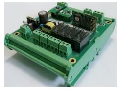
Step 4: Snap the housing onto 35mm DIN rail in your electric panel and wire accordingly.
