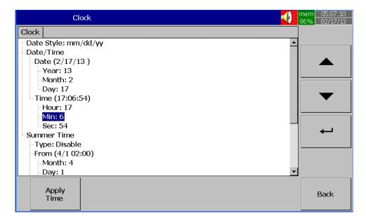
Fig: Clock configuration page in Paperless Recorder
