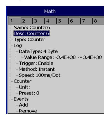
Press directional keys  $\langle \ \rangle$  at the bottom to select one of the Math channel for the Counter operation.
