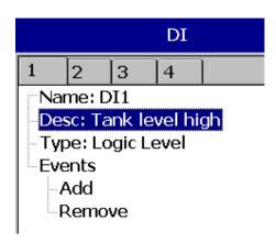
**Name**: Define the name for the Digital Input Channel. A maximum of 18 characters is allowed for the name.
