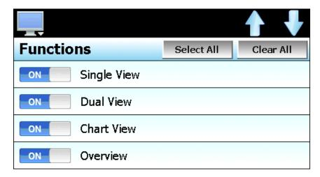
When functions are disabled at the configurator level from the **Functions** list, it will be disabled in the runtime software by removing the menu item so the operator can not select the function or edit any corresponding settings related to the function. The following list shows the available nCompass functions, where to find the menu item(s) applicable to the function and a description of what it applies to.
