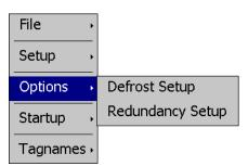
The **Options** menu provides access to additional controller options including the setup of defrost and redundancy operation.
