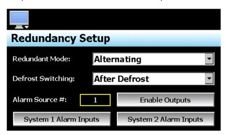
The **Redundant Mode** selection is used to choose how redundancy operates. Available selections are Disabled, Concurrent and Alternating. The concurrent and alternating redundancy modes select the back-up system mode of operation. When concurrent is selected, both system 1 and system 2 will operate at the same time when the selected alarm source in is alarm. When alternating is selected, nCompass will switch to the back-up system on alarm.
