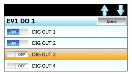
Select each output that is to be assigned to the event from the list and press the 'Done' button to assign the outputs to the event and return to the Event Setup screen.
