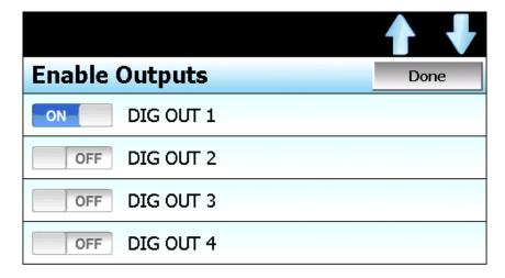
For example, if digital output 1 is used as the control output for the refrigeration system when a system event is turned on, then select digital output 1 from the list. This will enable the defrost logic whenever the refrigeration system is on. Additional outputs can be selected if necessary. Once all selections have been made, press the 'Done' button to accept the output selections and return to the Defrost Setup screen.
