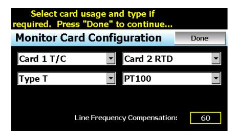
The card type drop down menu is used to select the type of monitor module connected to nCompass. Available selections are Not Used, Analog, RTD and Thermocouple.
