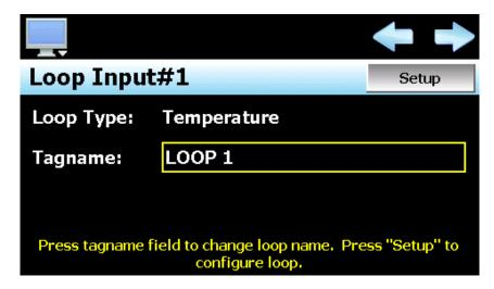
The left and right scroll (arrow) buttons allow the user access each loop in the system, by pressing left or right to go to the previous or next loop.
