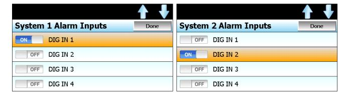
For example, if digital input 1 will be used for the system 1 failure input, then select digital input 1 from the list. If digital input 2 will be used for the system 2 failure input, select it as the alarm input for system 2. Additional inputs can be selected if necessary. Once all selections have been made, press the 'Done' button to accept the input selections and return to the Redundancy Setup screen.
