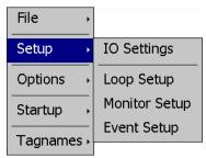
The **Setup** menu provides access to the primary controller setup options. These options include the number of loops and monitors used, the number of digital and analog inputs and outputs available, the number of alarms and events available as well as loop, monitor and event configuration.
