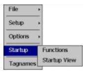
The **Startup** menu provides access to enable and disable nCompass runtime screens/menus and the select the desired startup view.
