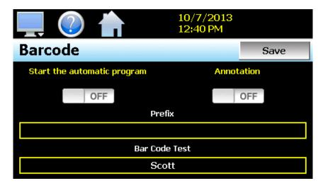
Barcode reader operation is enabled through the 'Start the automatic program' and 'Annotation' on/off buttons. The selections are mutually exclusive, i.e., only one can be enabled at a time. When one option is turned on, the other is automatically turned off.
