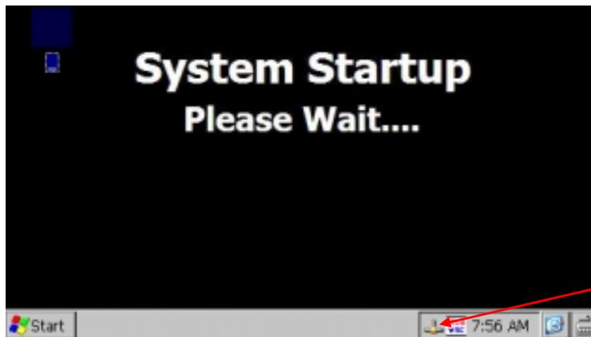
Next, double-tap on the network connections icon to open the network connection information window. Two tabs will be provided; one for IP Information and the other for IPv6 Information. To obtain the MAC address, press the 'Details...' button on the IP information tab.
