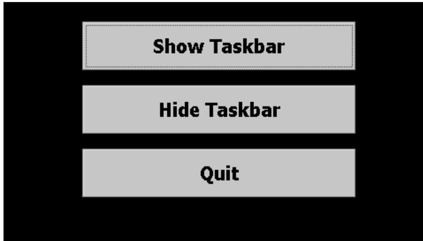
Press the 'Show Taskbar' button in order to show the taskbar and then press the 'Quit' button to exit the taskbar application. Before proceeding any further, enable the CE keyboard so that it will be available to enter in the IP address. If you do not enable it now, you will not be able to access the taskbar later once in the Ethernet Drivers screen.
