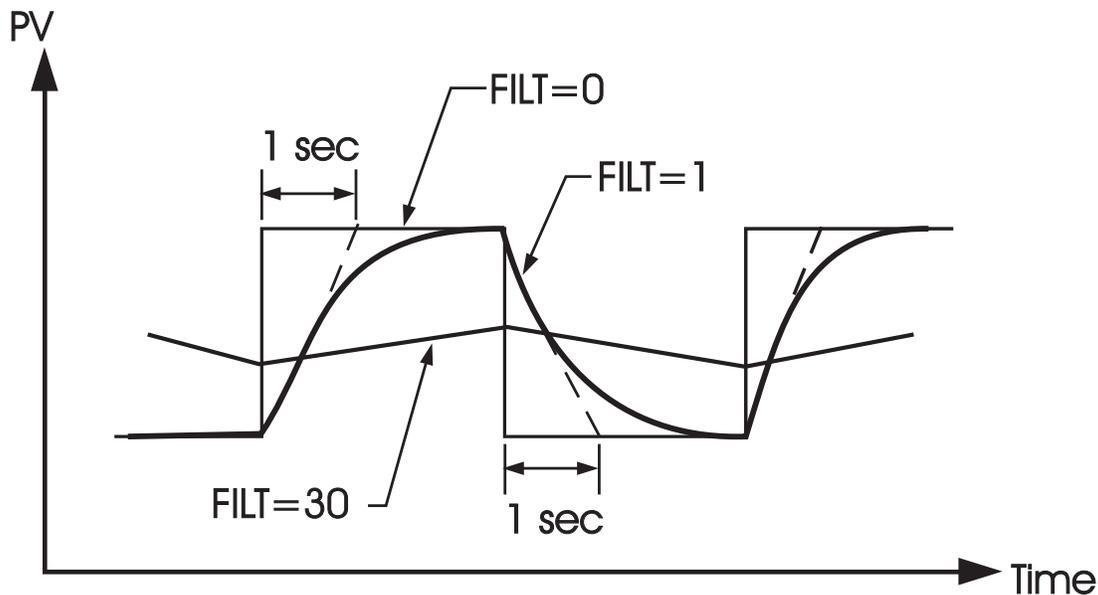
Figure 3.8 Filter Characteristics
