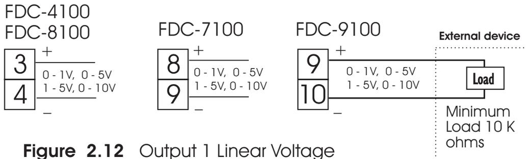
**Figure 2.12** Output 1 Linear Voltage
