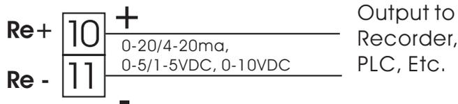
Load Resistance : 0 - 500 ohms ( for current output )
