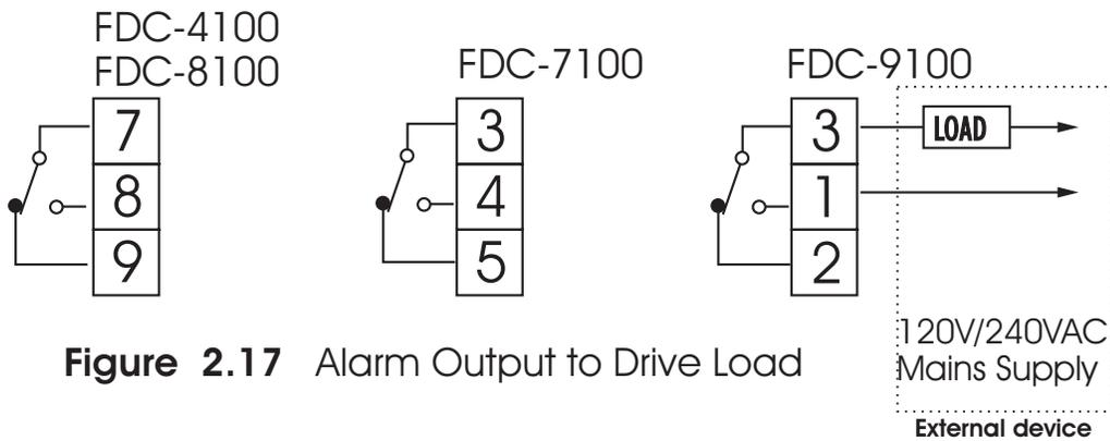
Figure 2.17 Alarm Output to Drive Load
