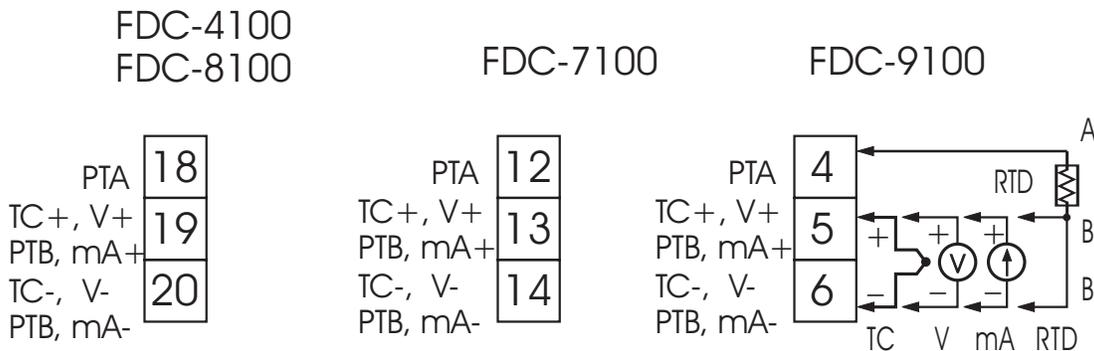
Figure 2.8 Sensor Input Wiring
