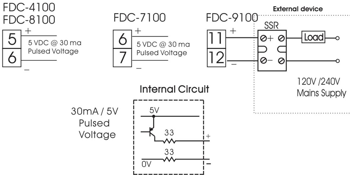
**Figure 2.14** Output 2 Pulsed Voltage to Drive SSR
