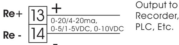
Load Resistance : 0 - 500 ohms ( for current output )
