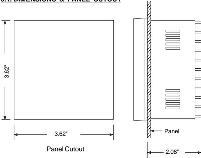
Figure 6.1. Mounting Dimensions
